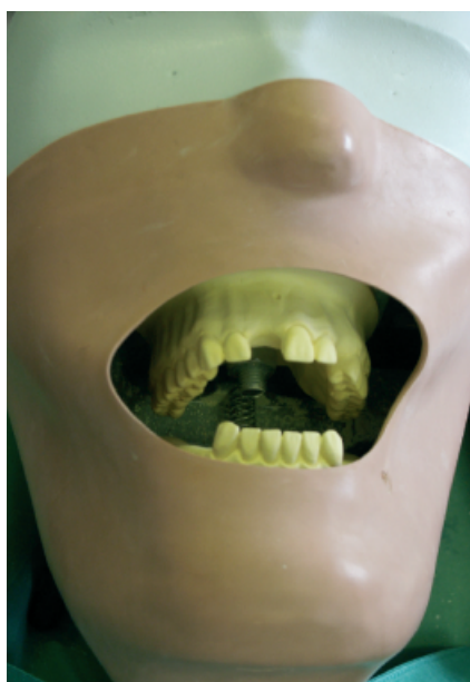
Fig. 1. In order to imitate the clinical application, all insertions were performed in a phantom head.
