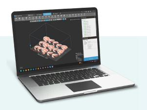
Create CAD files and import into 3D Sprint. Indicate shades, auto-position & support, and send to printer
