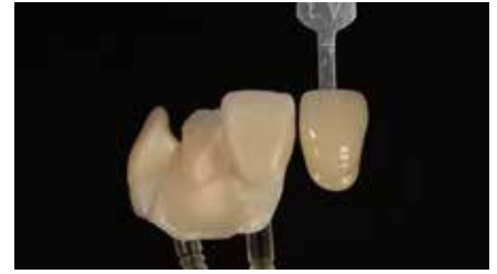
Fig. 10 After sintering with the simplest dipping technique: immersion in a single Body liquid
